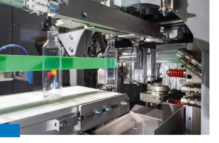
SIPA has introduced the SFL Flex machine, expanding its SFL range of linear stretch-blow molding machines to cater to the production of small batches. The SFL Flex is available in two versions, one with two cavities and the other with just one. These machines are designed for lower output segments, producing between 1000 to 4000 bottles per hour.
