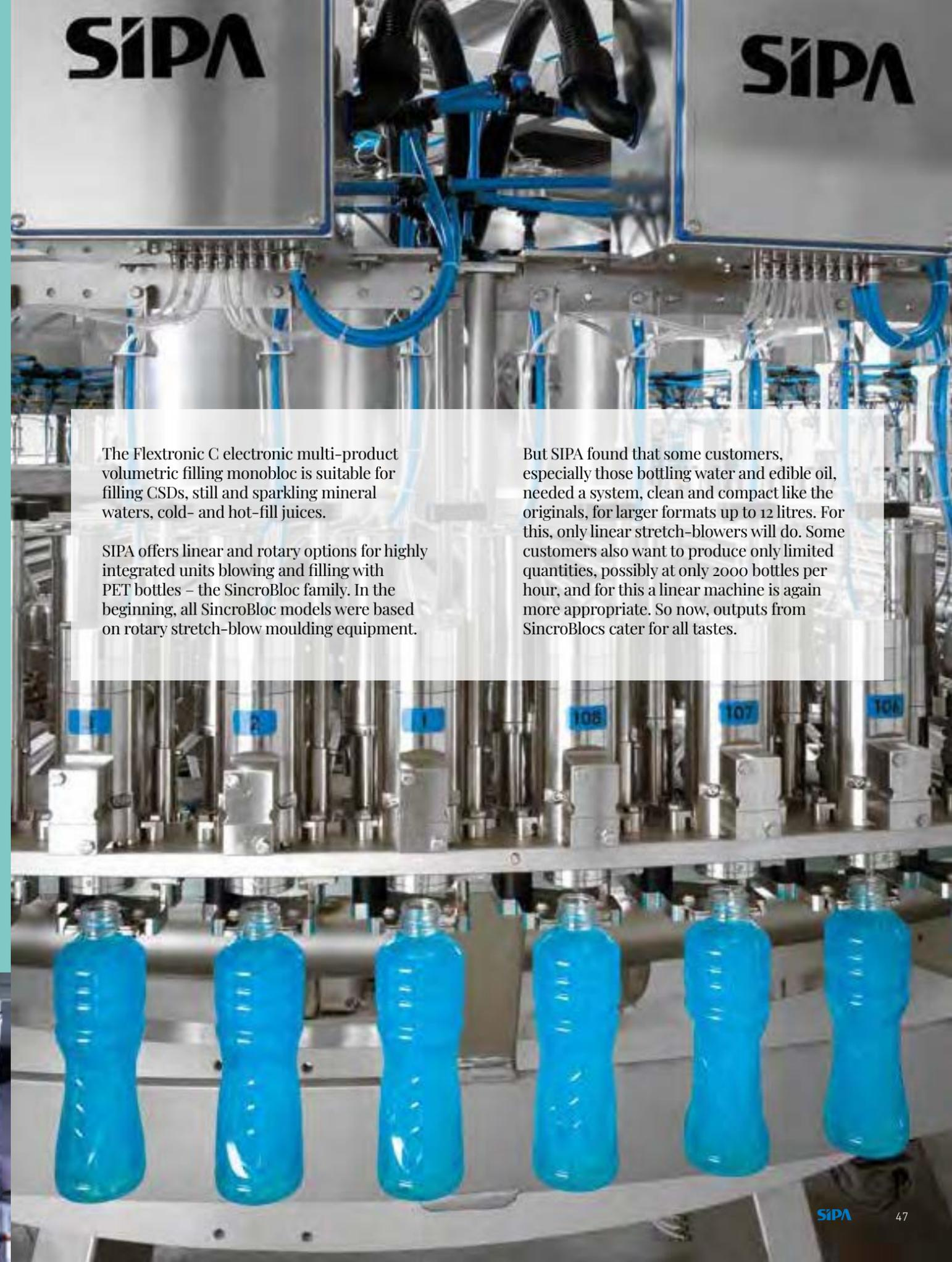
The Flextronic C electronic multi-product volumetric filling monobloc is suitable for filling CSDs, still and sparkling mineral waters, cold- and hot-fill juices.
