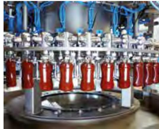
But they don't have to. SIPA has for some time been offering filling lines that can handle both types of product, with change-over times of just a very few hours. With SIPA's rotary stretch-blow molding machines and Flextronic C, the concept has even more added-value than ever. The ability to blow and fill diverse types of container on a single line has been made without compromising any performance characteristics of the line.
