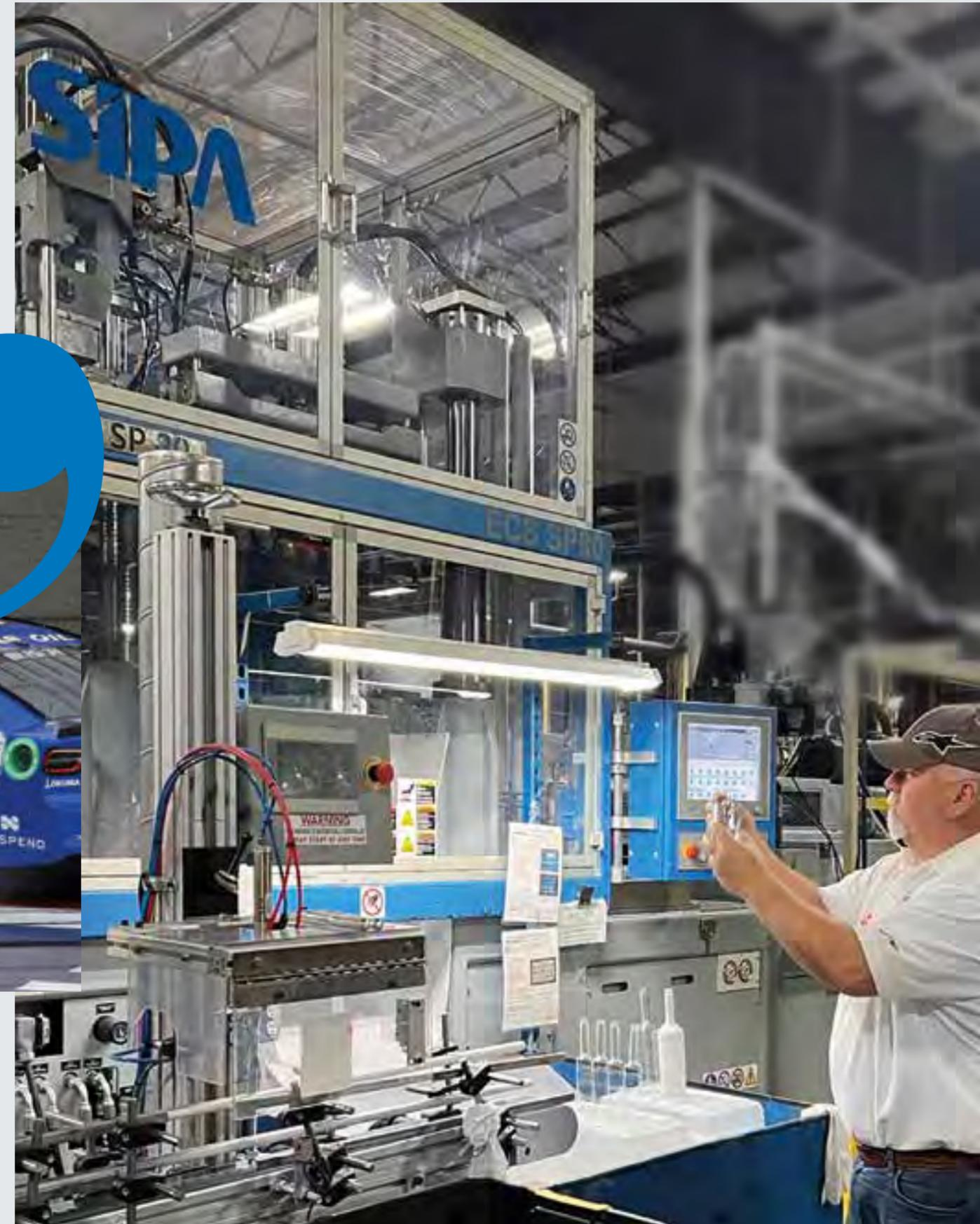
Single-stage production using the ECS SP 80 is ideal for these particular bottles, given the production numbers and the variety of sizes involved. The SIPA units run fast and efficiently, and the time and effort involved in changing format is low. The bottle maker can rely on responsive technical support from the people at SIPA North America, and that includes short turn-around times for any mold renovation or repairs.
