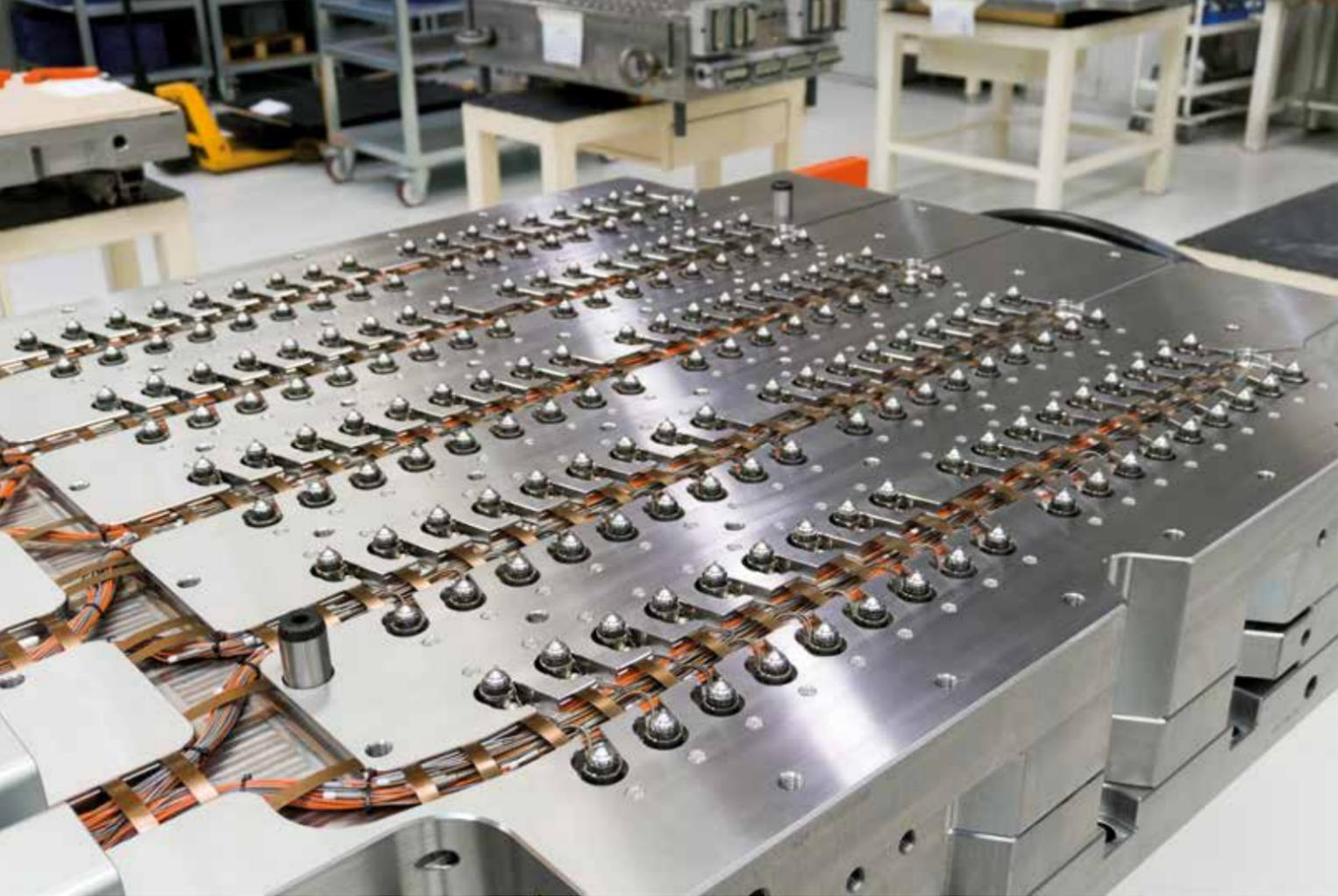
cylinders, making sure that any PET dust particles created in the system are evacuated every cycle. This solution should on its own be sufficient to keep the system clean. But just to be absolutely sure, there is also a “boost” function that can be activated to perform a forced cleaning cycle, at intervals that can be set by the user (every 40,000 cycles for example). This process lasts for a few tens of seconds, so it has no impact on productivity.
