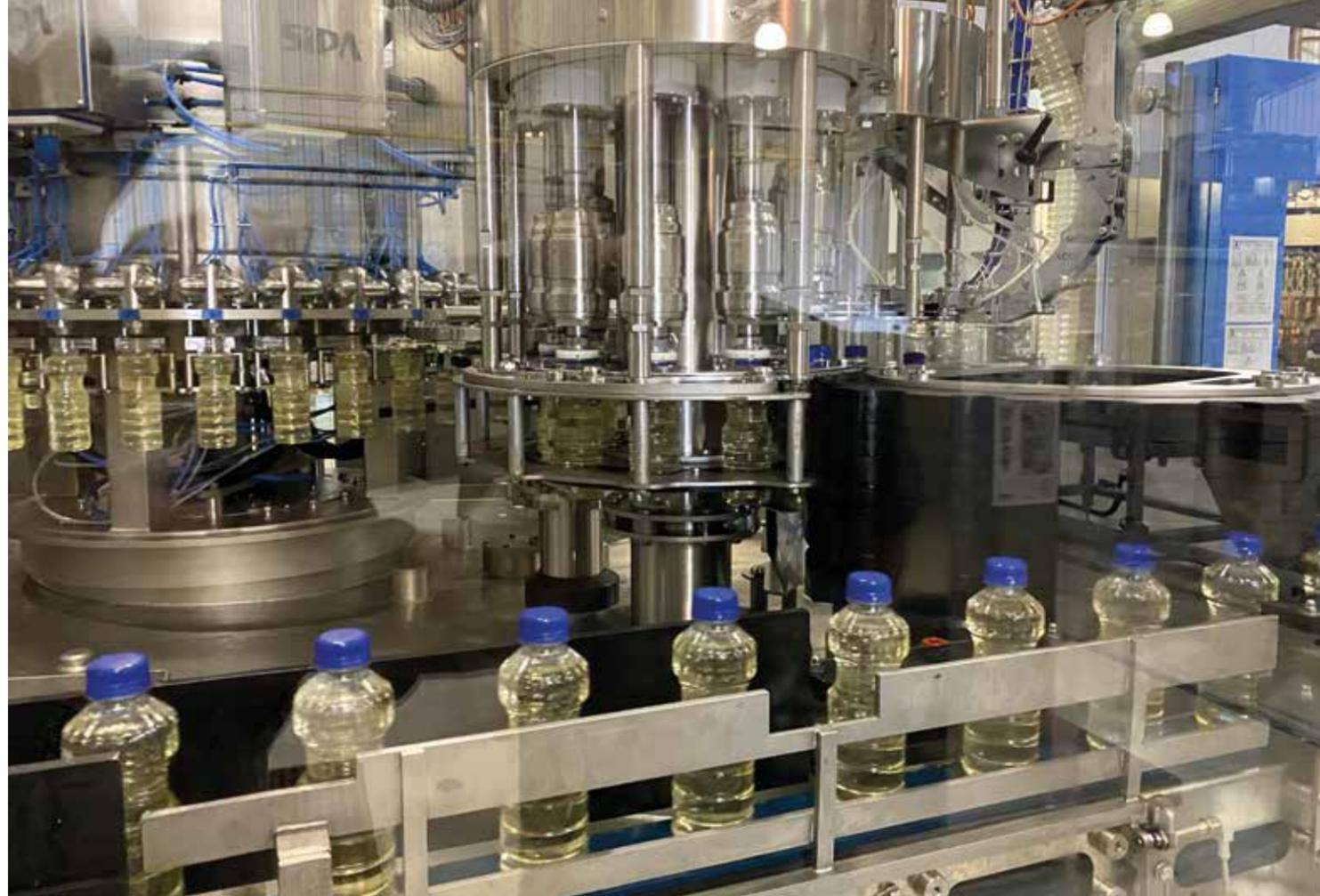
The Sincro Bloc system features very fast product changeover without the need for special tools. The line is equipped with an ECHO system for remote control and monitoring, enabling digital management.
