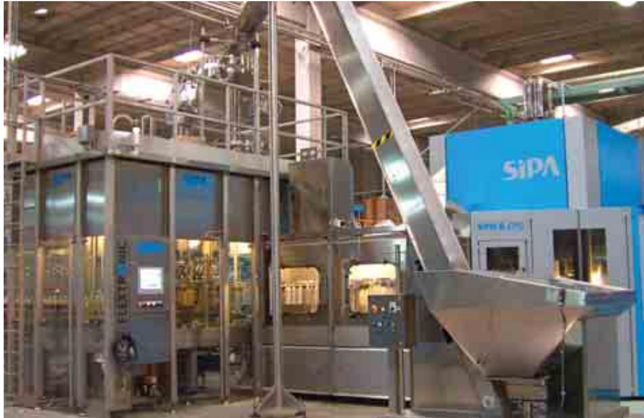
The Flextronic W is highly suited to lightweight bottles, as it handles them only by the neck. It also comes with the option of pressurizing the bottles with nitrogen in order to prevent the oil inside from oxidizing and losing its flavor. "Aceitera Martinez was very happy with the first line we installed, so it quickly chose the
