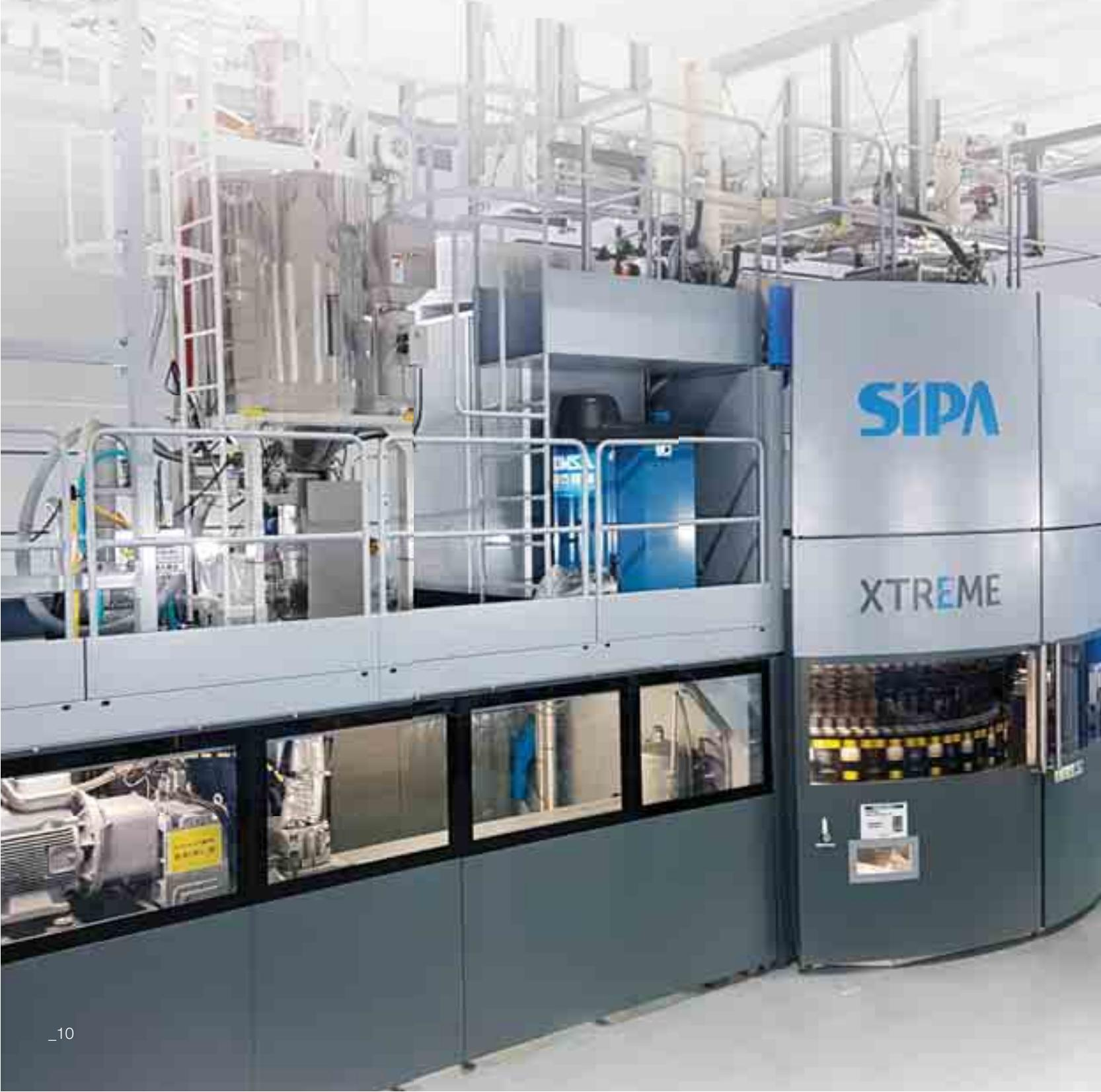
that used in conventional injection molding. The low-pressure production of preforms enables a weight reduction in every preform compared to the lightest injection molded preforms on the market today, creating important savings in production costs and, most importantly, in the amount of PET used thus reducing the environmental burden such as CO<sub>2</sub> emissions.
