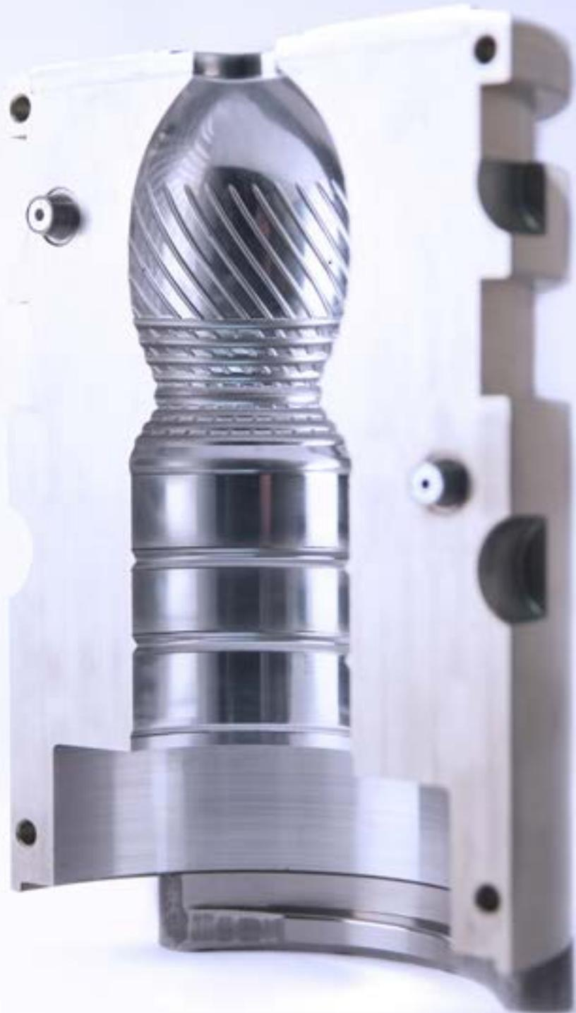
and the two body mold halves, but these fissures on their own are not enough. For this reason, virtually all molds now incorporate numerous venting holes in well-defined positions to allow the passage of air to the exterior of the mold.
