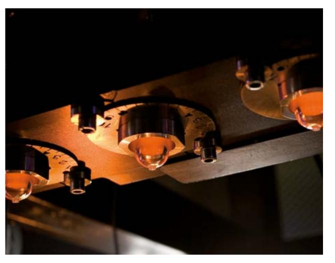
just below the preform neck, while protective shields prevent the body from heating up. Ths system therefore works without any need for the bottles to rotate, making the process more reliable and efficient, with longer maintenance intervals.
