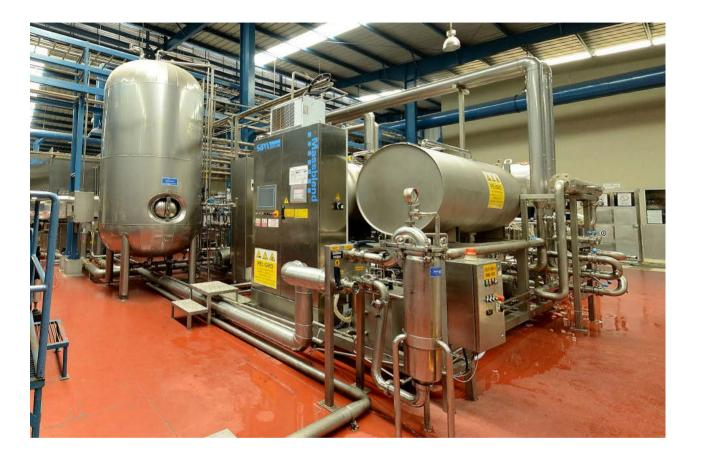
pneumatically operated transport system. The filling line itself comprises an ISOFILL isobaric filling monoblock, a DRINKMIX continuous mixing unit, labelling and bundling units from SIPA partners in Italy, and a FASTLAYER palletisation system.
