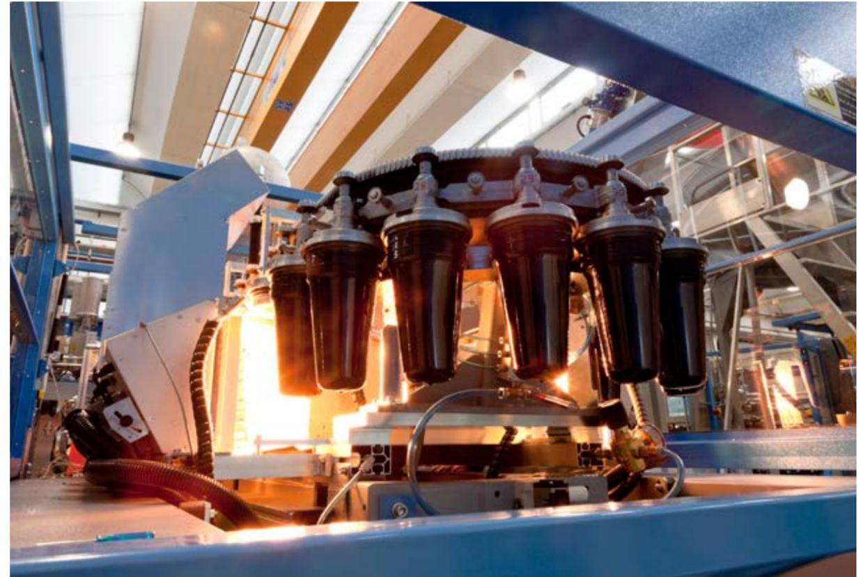
SIPA's very broad range of stretch-blow molding machines caters for diverse customer needs in terms of output rates and container size; there is of course also the choice between linear and rotary machines. One especially versatile model is the linear SFL 4/3 XL, with its ability to hold one, two, or three cavities (format changes are quick and simple to carry out) and to produce containers as small as 12 mL and as large as 12L, at speeds of up to 5400 bottles per hour.
