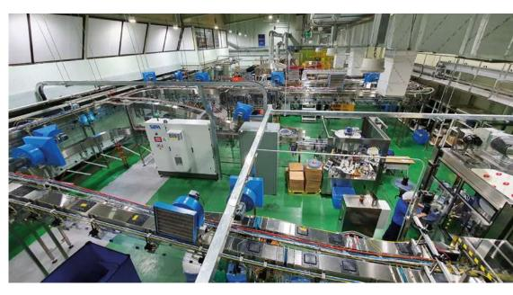
Bottles are blown on a previously acquired stretch-blow molding unit. They are then sent via a SIPA air conveying system to the labelling/filling/capping/inspection/shrink wrapping/palletizing/pallet wrapping line, again completely installed by SIPA. Larger bottles also have handles automatically attached to them – once more, using equipment installed by SIPA.
