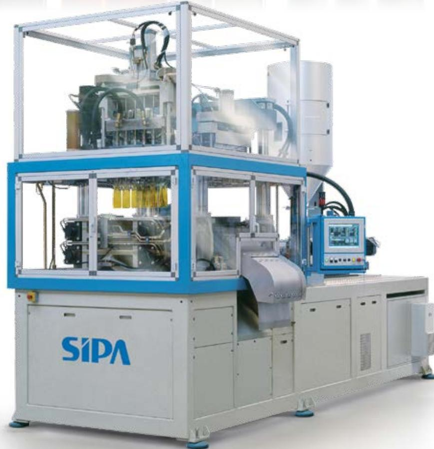
vider to introduce the amorphous reinforced neck for hot fill applications without the need of the traditional crystallized neck, thus reducing dramatically the container production cost.
