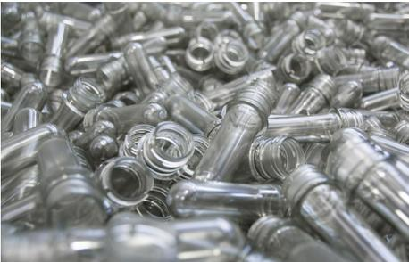
Picture 3: The PET Inline Preform system enables the flexible direct processing of PET flakes to make food contact compliant inline preforms in just one processing step.
