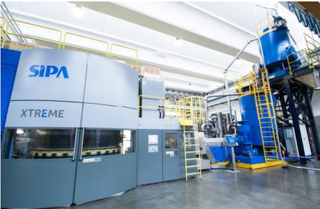
Picture 2: The new PET Inline Preform system combines the efficiency benefits of the proven VACUREMA technology from EREMA with the innovative XTREME preform production system of SIPA.
